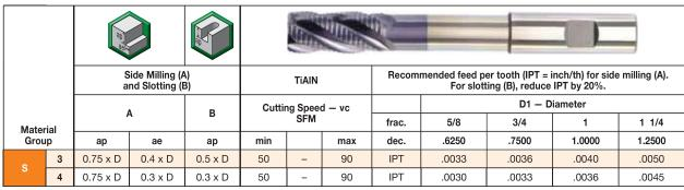
NOTE: Side milling applications — For longest length tools, reduce ae by 30%.
